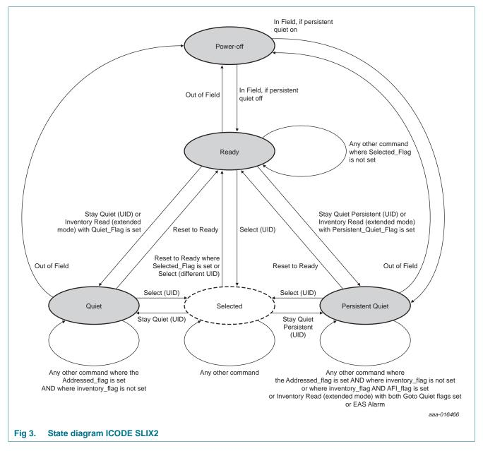
**Remark:** It is possible to set the ICODE SLIX2 IC into the Quiet and Persistent Qiet.mode at the same time. In this case the behavior is the same as for the Quiet state only until the IC enters the Power-off state. The IC enters to the Persistent Quiet mode at the next power-on if the persistent time has not been exceeded.
