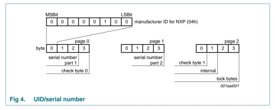
According to ISO/IEC14443-3 BCC0 is defined as  $CT \oplus SN0 \oplus SN1 \oplus SN2$ . Abbreviations CT stays for Cascade Tag byte (88h) and BCC1 is defined as  $SN3 \oplus SN4 \oplus SN5 \oplus SN6$ .
