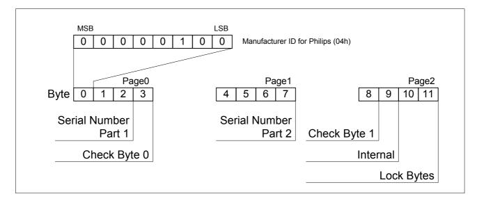
According to ISO/IEC14443-3 Check Byte0 (BCC0) is defined as  $CT \oplus SN0 \oplus SN1 \oplus SN2$  and Check Byte 1 (BCC1) is defined as  $SN3 \oplus SN4 \oplus SN5 \oplus SN6$ .
