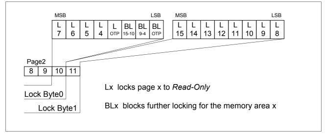
9 to 4 and bit 0 page 3 (OTP). Once the block-locking bits are set the locking configuration for the corresponding memory area is frozen.
